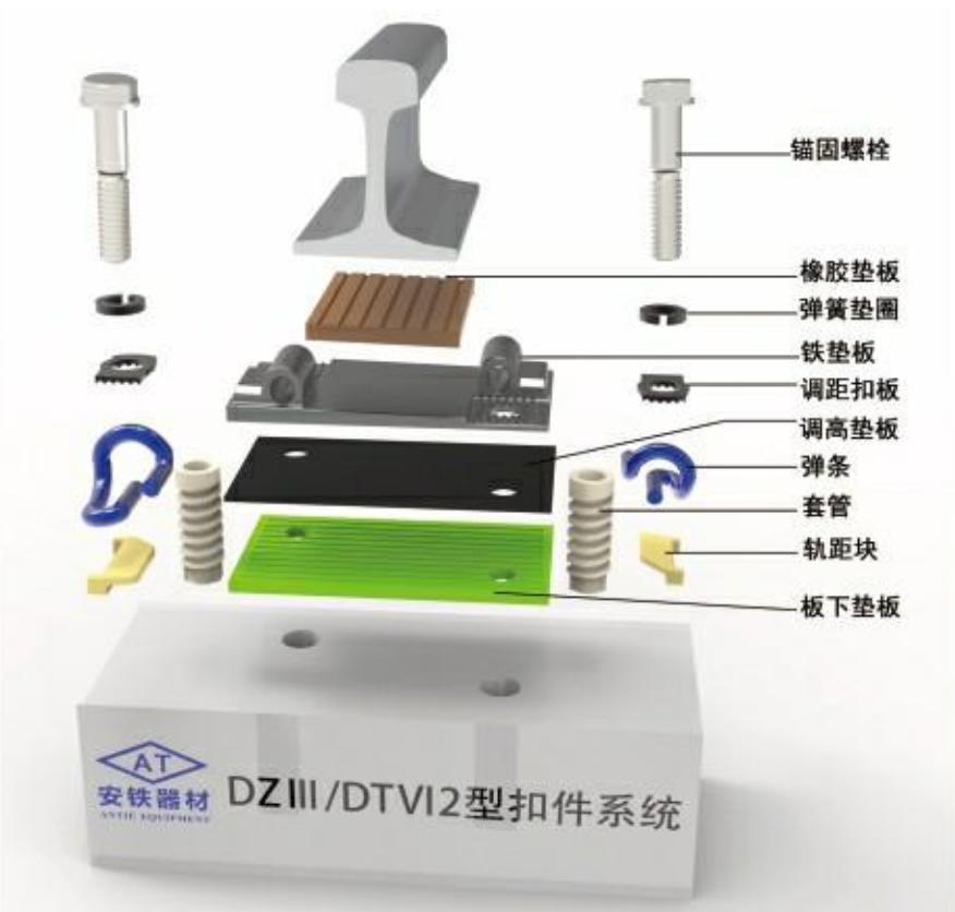
地铁DZIII, DTVI2扣件 DZIII, DTVI2 Fastening System
